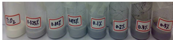
Figure 2: Snapshot of nanocomposite paste of MWNTs-MA/TiO 2 of various CNTs weight percent
