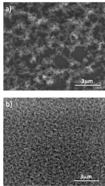
Figure 1: SEM images of ormosil thin films prepared by using gels synthesized in different solvents (a) methanol, (b) DMSO.
