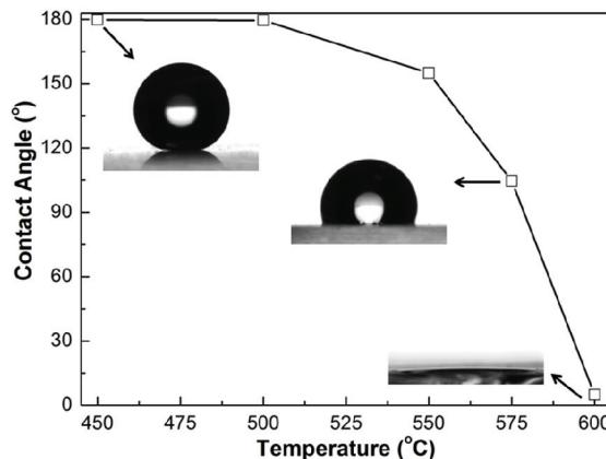
Figure 3: Water contact angles of annealed ormosil films at different temperatures.
