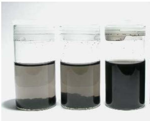
Figure 2: Photographs of dispersions of carbon nanotubes in DMF after 5 min of mild sonication and settling overnight. Left to right: as-grown nanotubes, 3 cycles of thermal cutting, 6 cycles of thermal cutting.
