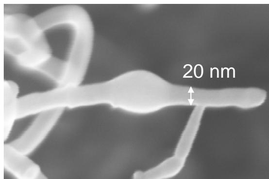
Figure 3: Scanning electron micrograph of a polymer droplet on a carbon nanotube. The shape of the droplet can be used to calculate the contact angle.
