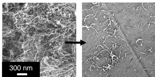
Figure 1: Scanning electron micrograph showing the effect of cutting the original entangled nanotubes (left) into shorter fragments (right)
