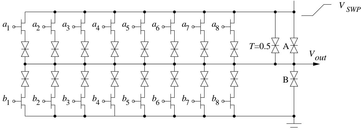
Figure 5: A configurable pattern matching circuit to match two 8-bit patterns with any error tolerance from 0 to 8. Note that the threshold RTD has half the area as that of all other RTDs and may be combined with RTD A.
