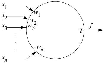
Figure 1: Representation of the threshold function  $f$ .
