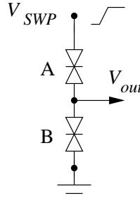
Figure 4: Schematic representation of a MOBILE.
