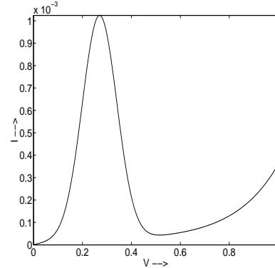
Figure 3:  $I - V$  characteristics of a RTD.
